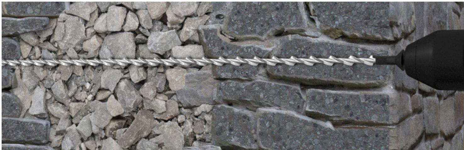
Thor Helical ties are particularly useful for tying rubble filled walls. The helical wall tie bars connect the inner and outer layers of old stone walls in situations where the core between them is filled with rubble or other infill.
